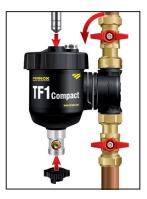
4. Close drain valve, replace magnet and open inlet valve
