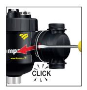
Using a flat end screwdriver in the recess shown, gently lever the locking clip into the 'unlock' position.
