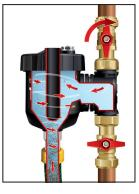
3. Open outlet and drain valves
